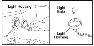
To replace the light bulb, pull the old light bulb out of the housing and insert a new light bulb. Re-attach the light housing to the spa shell. Re-attach the access panel to the spa.
